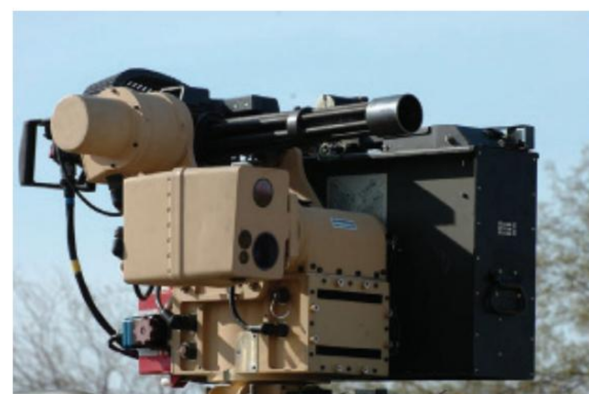
RWS fitted with Dillon Aero M134-Series minigun
